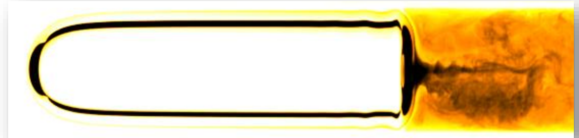
Reactive Oxygen Taylor Bubble - Solution of Cu(btmgp)I (20 mM) in Acetonitrile at ambient pressure and temperature. Source: Project Group Prof. Dr.-Ing. Michael Schlüter, TU Hamburg: Experimental Investigation of Reactive Bubbly Flows - Influence of Boundary Layer Dynamics on Mass Transfer and Chemical Reactions
